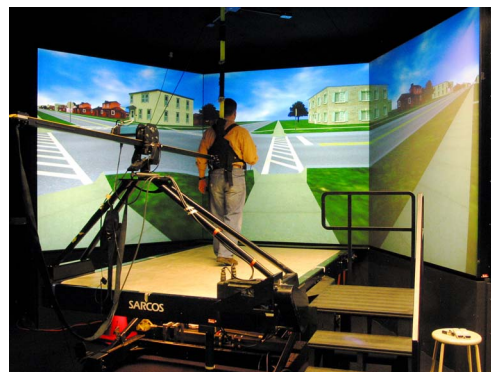
Figure 1 Treadport Virtual Environment comprising a CAVE-like visual display and locomotion interface
