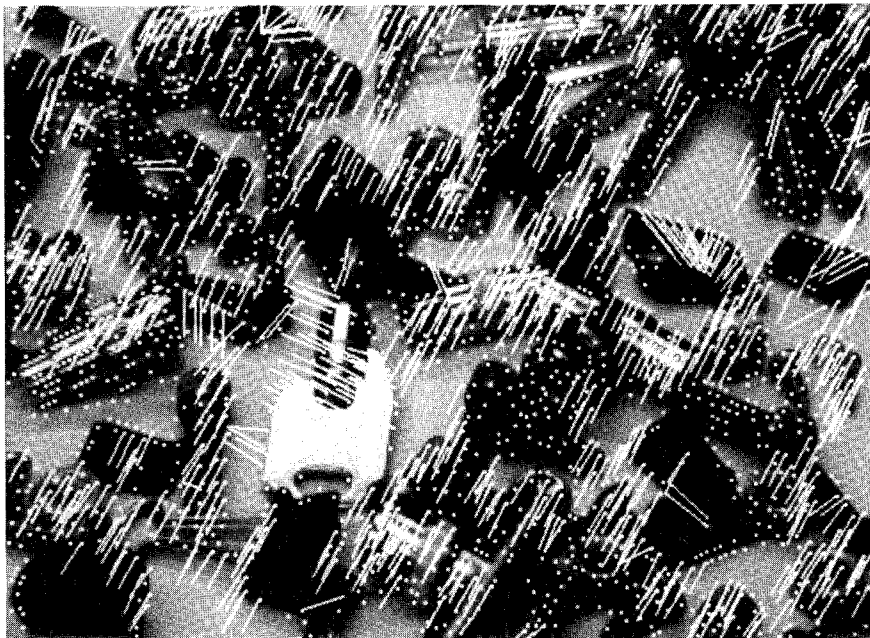
Fig. 14. Optical flow field obtained from the image sequence of figure 13.
