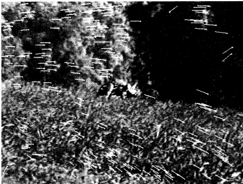
Fig. 9. Optical flow field obtained from the image sequence of figure 8.
